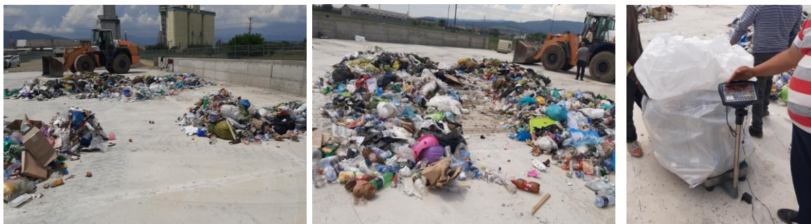
Figure 80 General characterisation; a) piles of different fractions; b) mixing and splitting waste for preparing samples; c) weighing different components
