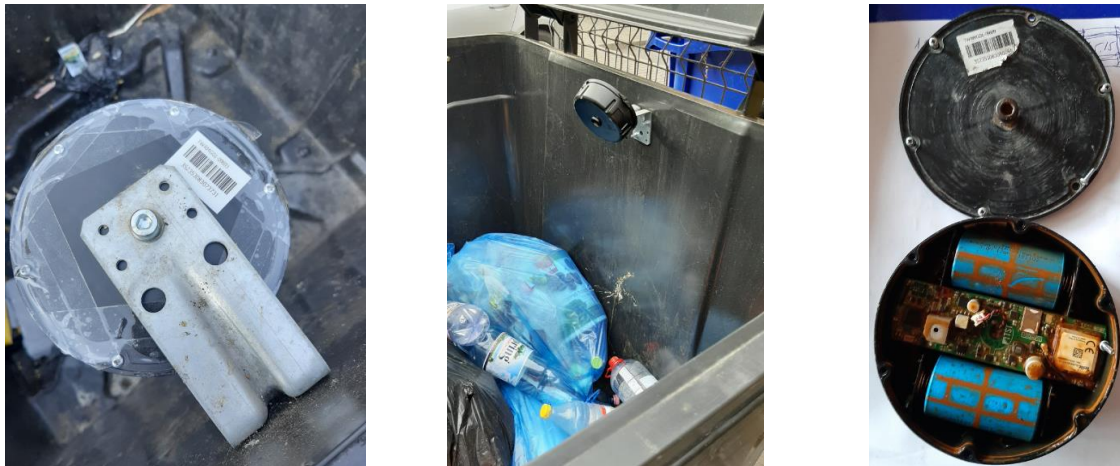
Figure 55 Filling sensors; a) Supplementary insulation; b) Forced (tilting) sensor bracket; c) Sensor with water inside
