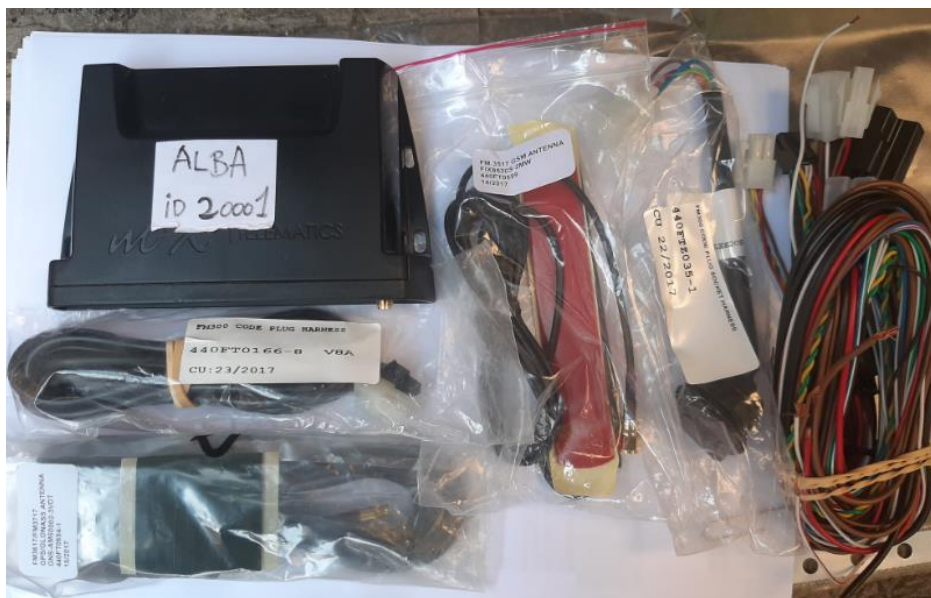
Figure 12 CAN-BUS kit prepared for installation on dedicated truck in Alba Iulia
