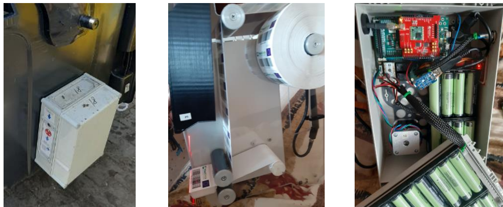
Figure 8 Identity module: a) appearance; b) indoor - label roll and reader; c) batteries and electronics
