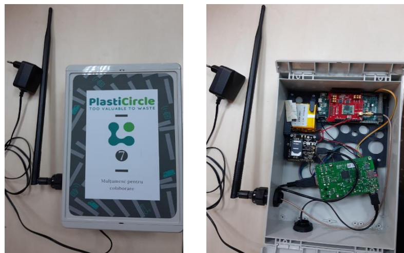
Figure 9 Local transceivers prepared for Alba Iulia, included high gain antennas in order to improve coverage; a) outside; b) inside electronics
