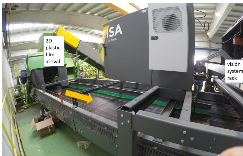
Test Center 2D plastic film sorter
